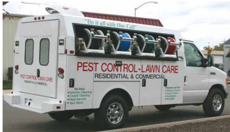
Six Tank, 3 Pump Multi-purpose Van System
