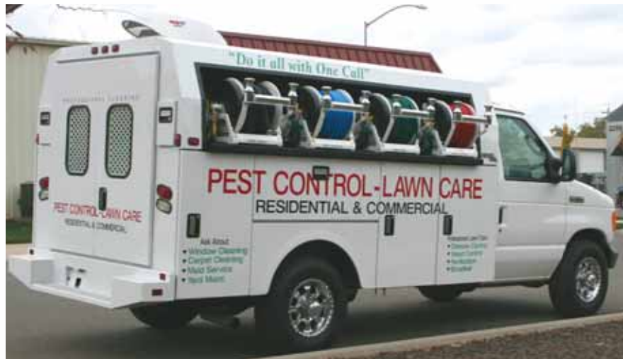
Six Tank, 3 Pump Multi-purpose Van System
